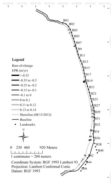
**Figure 8.** Long term annual rate-of-changes for Almanarre Beach (Negative and positive values indicate erosion and accretion, respectively)
