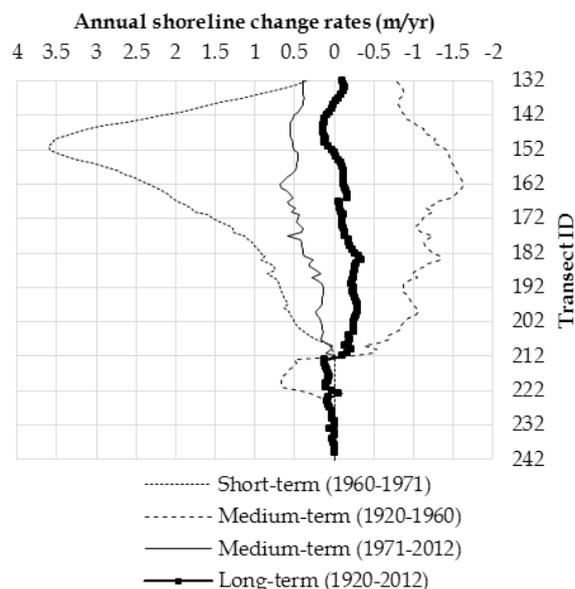
**Figure 7.** Short, medium, and long term annual shoreline change rates in the sector 4 of the Almanarre Beach (Negative and positive values indicate erosion and accretion, respectively)
