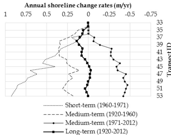
**Figure 4.** Short, medium, and long term annual shoreline change rates in sector 1 of the Almanarre Beach (Negative and positive values indicate erosion and accretion, respectively)
