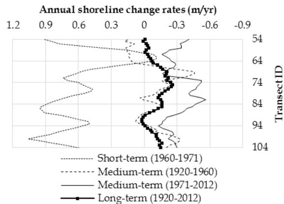
**Figure 5.** Short, medium, and long term annual shoreline change rates in sector 2 of the Almanarre Beach (Negative and positive values indicate erosion and accretion, respectively)
