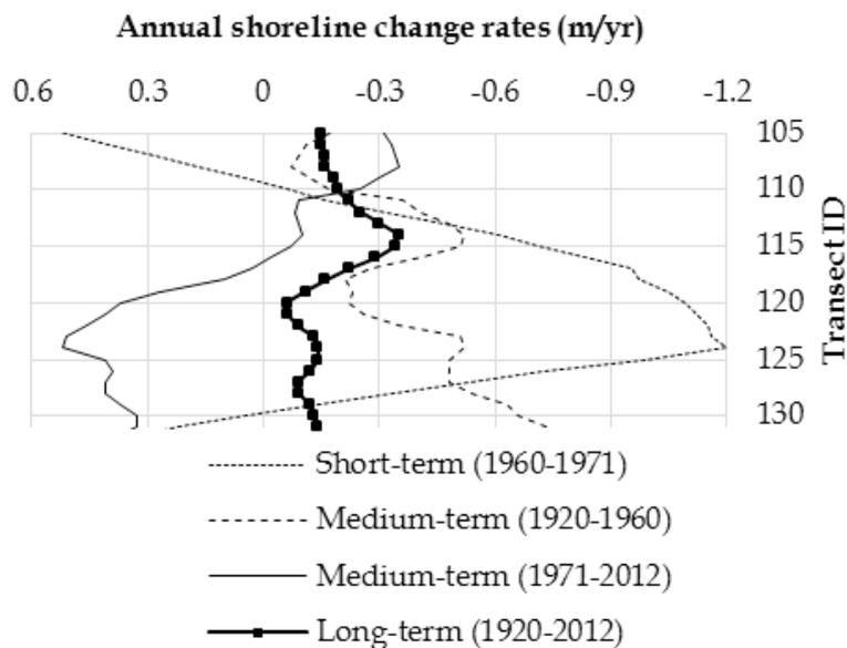
**Figure 6.** Short, medium, and long term annual shoreline change rates in sector 3 of the Almanarre Beach (Negative and positive values indicate erosion and accretion, respectively)
