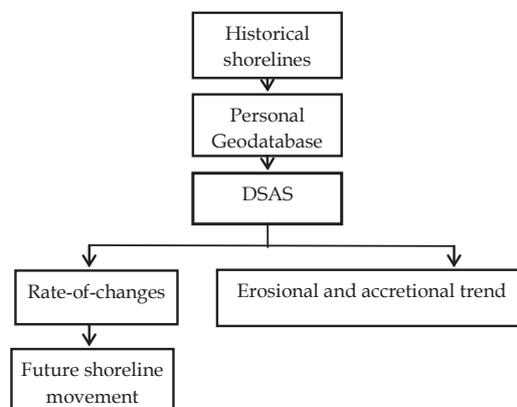
**Figure 2.** Workflow for the rate-of-changes estimation and prediction of shoreline changes
